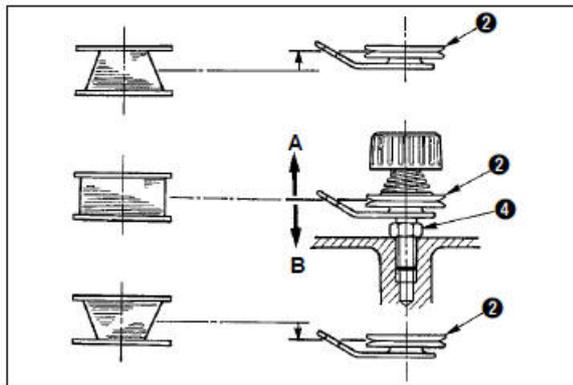
6 ) If user can not wind the thread smoothly, user should loosen the nut ○,4, turn the winding tension device and adjust the height of the thread tension plate○,2.
