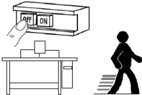
3、 If user needs tilt the head or replace the needle or thread the upper thread, please turn off the power
