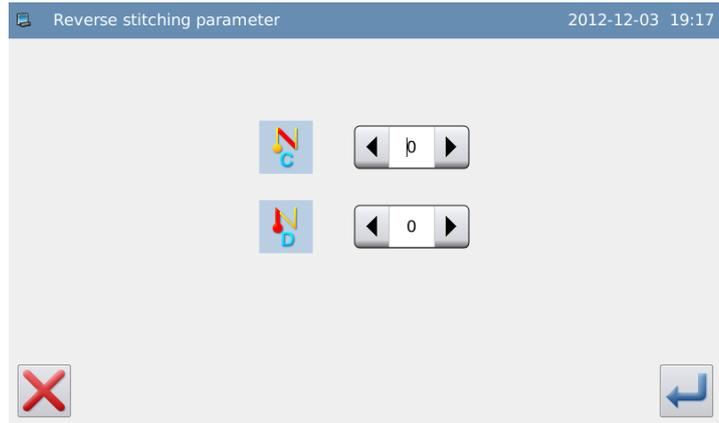
The width adjustment can narrow the distance from the original needle entry point to the next needle entry point at reverse sewing (no adjustment when the value is 0)
