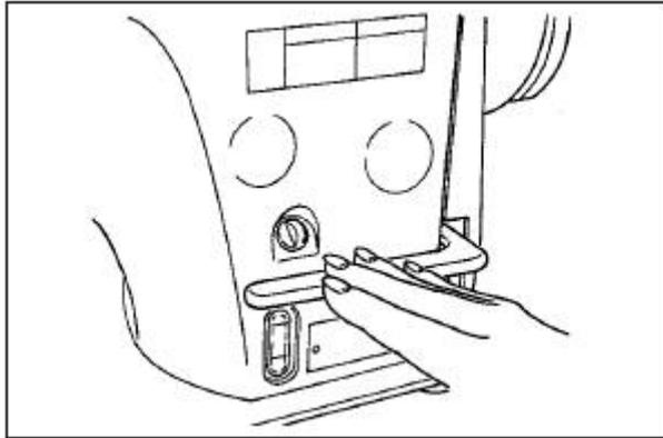
The contraction sewing is to operate the feeding bar to reduce the feeding interval to stop sewing at the sewing start or sewing end.
